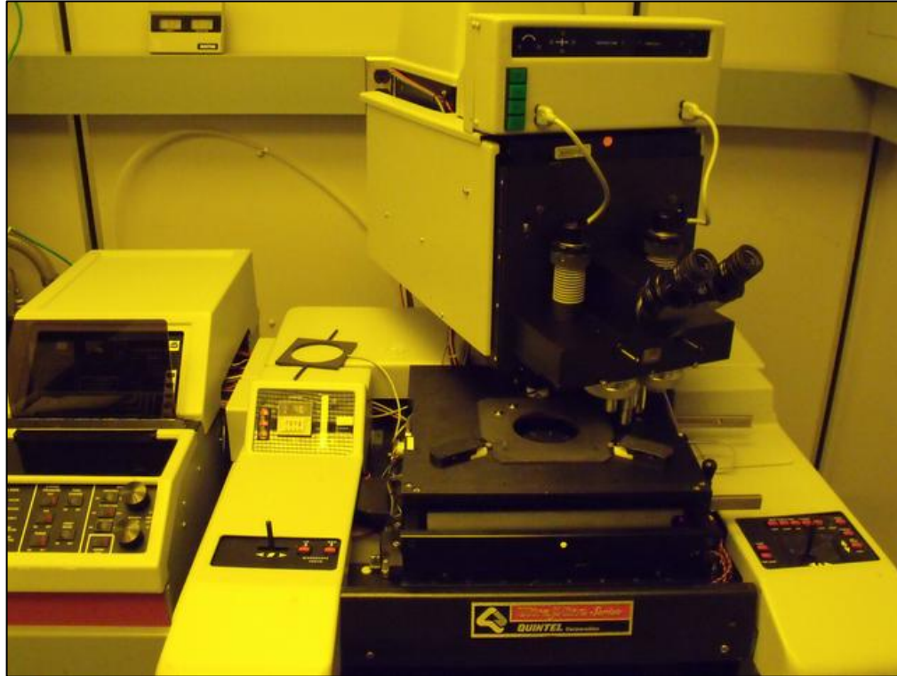
A typical contact aligner
